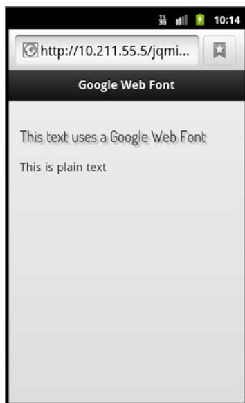
FIGURE 14.4 Using a custom font on a mobile browser with Google Web Fonts
