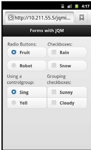
FIGURE 10.4 Radio buttons and check boxes displayed with and without a control group
